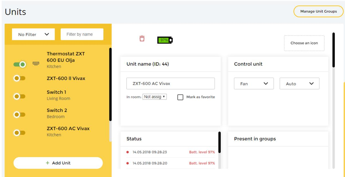
In the field Filter by name add a name of any installed device or in this example Switch. The application will automatically refresh the units, and only units that contain switch in the name will appear.
